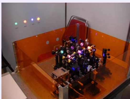
Fig. 1: Picture of Pr:YLF lasers pumped by 500mW GaN LD. Three cavities designed for 635, 607, and 522 nm show lasing
